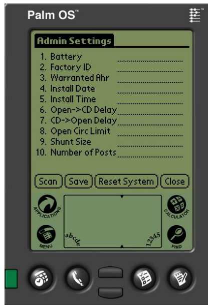
Fig. 5: Typical Palm screens showing installation data as well as the Warranted Amp-Hours
